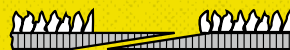
Type 5 Overlapping glued joint. Grit zone is completely ground off. Preferred joint for wood finishes with flat contact elements.
